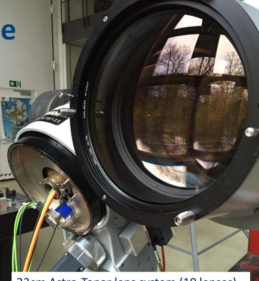
33cm Astro-Topar lens system (10 lenses), FoV w/ 10k×10k CCD: 52 deg<sup>2</sup>, 2.47"/px
