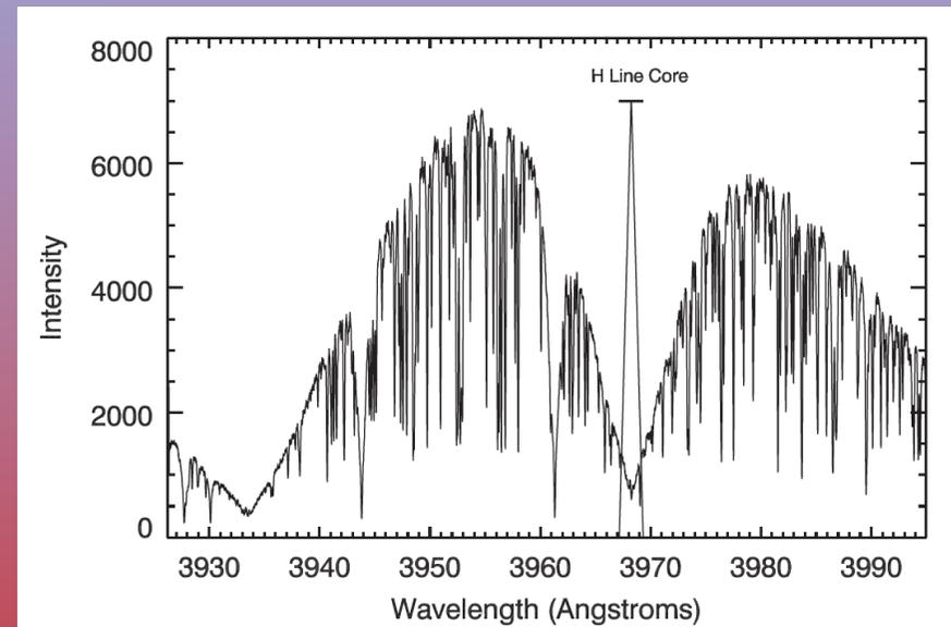
**Width of line core: 0.2 nm --> 150 km/s --> 70 pixel with PLATOspect**
