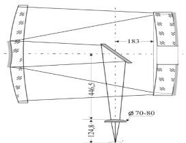
Limiting magnitude: ~ 12<sup>m</sup> The optical layout: Catadioptrical **Field-of-view**: 11.1' x 8.3' **Photometry acquisition:** the most active photometric telescope
