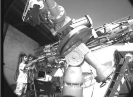
Light sensor: High speed photometer based on PMT FEU-79 with Johnson-Cousins UBVRI color filters system
