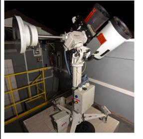
**TAL-250K** Location: Mayaki Main mirror diameter: 250 mm Focal length: 2130 mm Focal ratio: F/8.5 Limiting magnitude: 14<sup>m</sup> **Field-of-view:** 33' x 13' Camera: FLI ML8300
