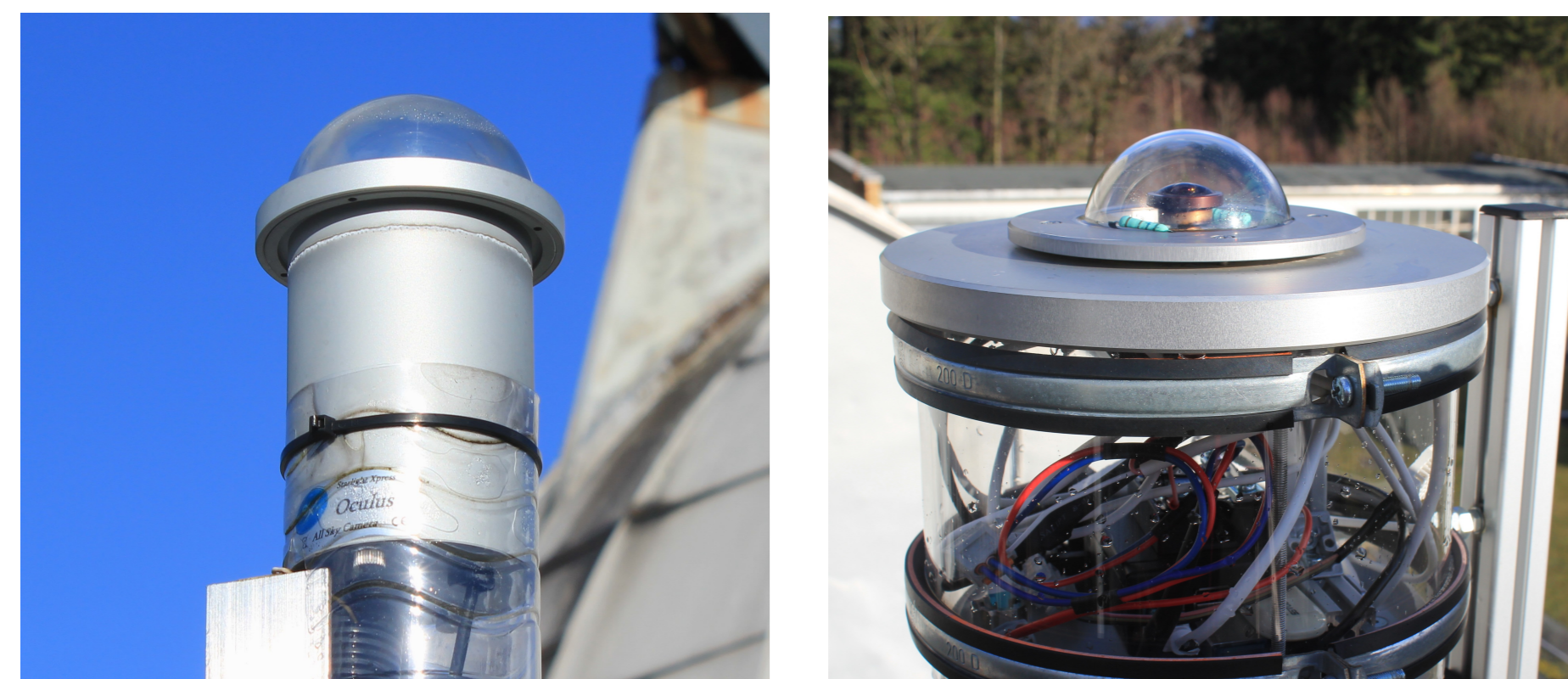
Figure 1: Starlight Xpress Oculus (left) and in-house developed fish-eye camera (right) set up on the roof of main building.
